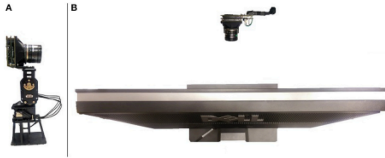
Figure 3.3: (A) A picture of the ATIS mounted on the pan tilt unit used in the conversion system. (B) The ATIS placed viewing the LCD monitor.[12]
